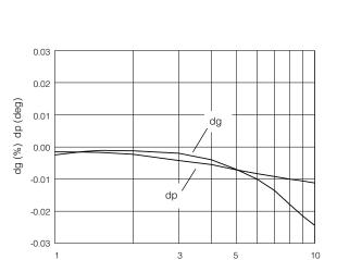
Fig. 6 Differential Gain and Phase vs Frequency
