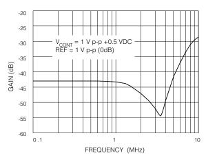
Fig. 4 Crossfade Balance vs Frequency
