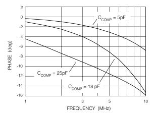
Fig. 5 Phase Delay vs Frequency
